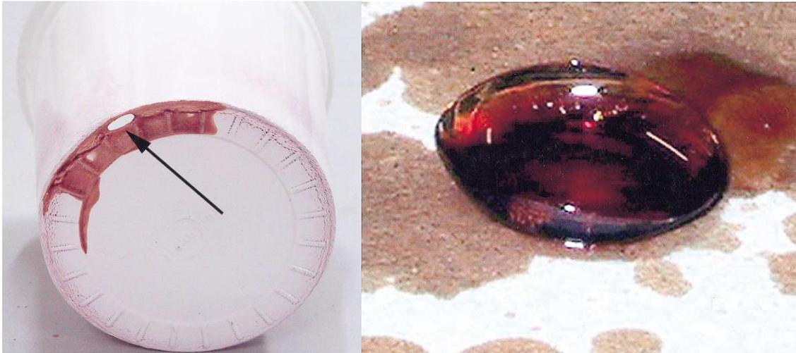
**Figure 17:** Hole in a plastic cup (left) and hardened stained contact lens (right) after OC
